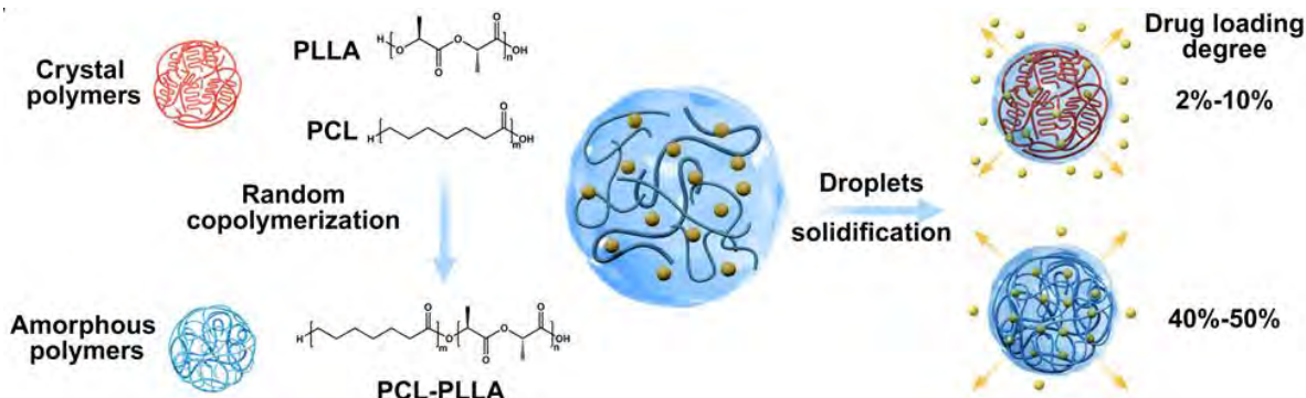
Fig. 1 Influence of the crystallization property on the droplet solidification and drug loading degree.
